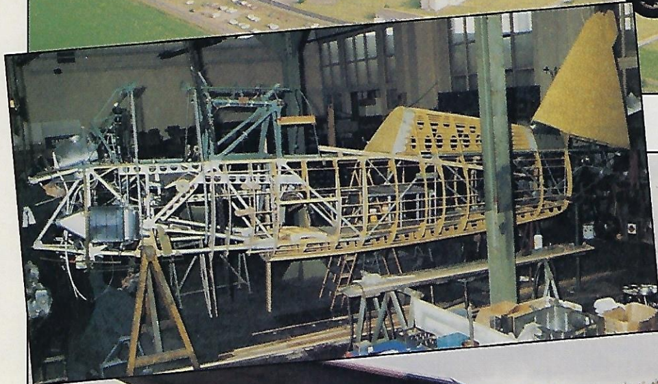
Airframe of Lysander Mk. III RCAF s/n 2442 beginning to take shape.
