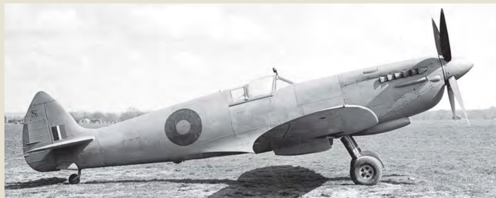
ABOVE: The PR.X was externally similar to the Mk.XI, but had a pressurised cockpit as shown by the cabin air intake below the exhaust and heavier canopy slide rails. The type entered service in the spring of 1944
