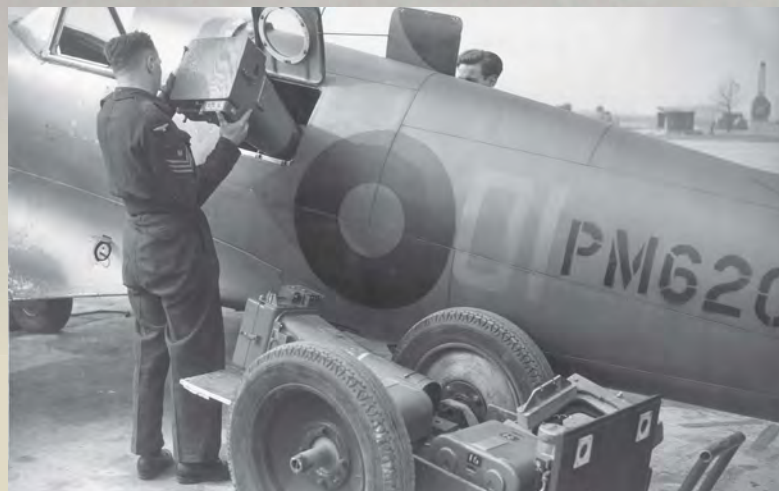
LEFT: Two long-focus F.52 cameras are inserted into the fuselage of 2 Squadron Spitfire PR.XIX PM620. The cameras were remotely controlled by the pilot, the downwards-looking installation in the Mk.XIX proving to be highly successful
