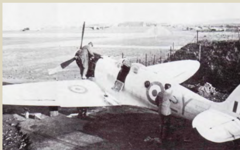
LEFT: Not all recon Spitfires were unarmed. Seen at RAF St Eval in Cornwall, pink-painted PR.Ig R7059 carried the usual Spitfire Mk.I armament of eight .303in machine guns in the wings, with its cameras mounted in the fuselage. This mark was later redesignated as PR.VII MALCOLM V LOWE COLLECTION
