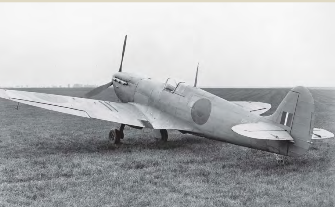
BELOW: Reinforcing strips on the upper wing surface are evident in this view of a production Spitfire PR.Mk.IV. Originally the Mk.I PR Type D or PR.Id, this version featured extended range and was a valuable addition to the growing selection of recce sub-types
