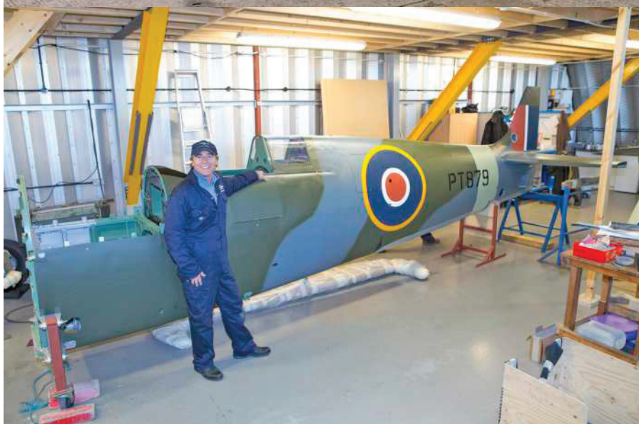
Teichman with the fuselage after painting. The decision was made to paint the aircraft as it had left the factory and then apply the Soviet markings over the British insignia. Little did the collector realize the Mk. IX would occupy two decades of his life.
