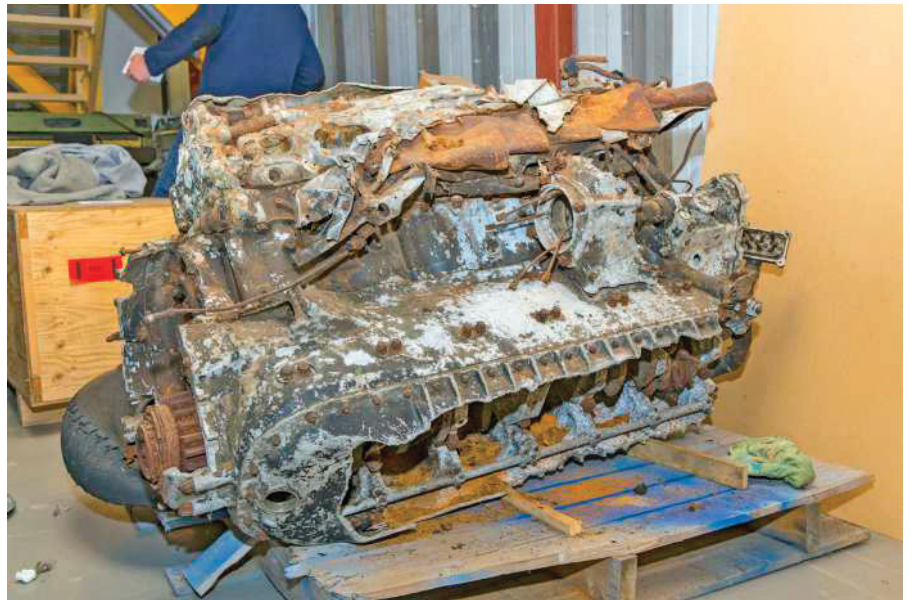
The original Rolls-Royce Merlin 66 was destroyed on impact with the tundra. Another variant would have easily fit the Mk. IX but Peter Teichman is a perfectionist when it comes to the Spitfire and he decided to go on the hunt for a replacement Merlin 66. It wasn't easy.
