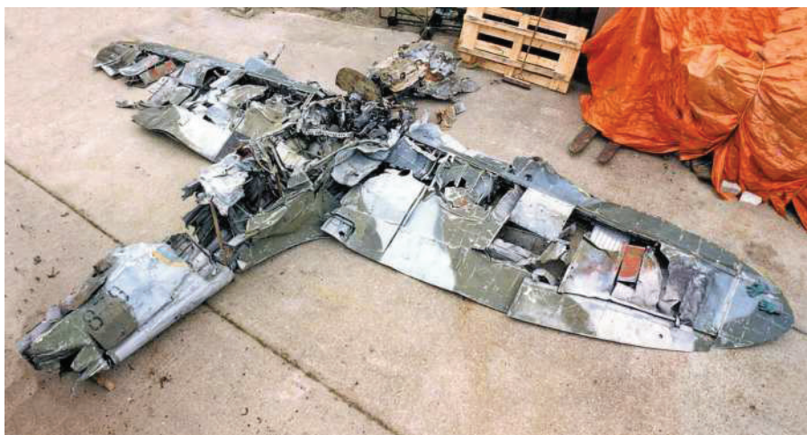
This is how the wreck looked after it was recovered. Note the missing tail. The pilot bailed out after PT879's tail was cutoff in a mid-air collision with another Spitfire. As can be seen, it appears the fighter impacted the tundra while in a near-flat spin. (Peter Arnold)
