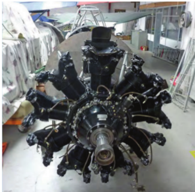
A head-on view of the restoration, showing the project's original Cyclone engine.
